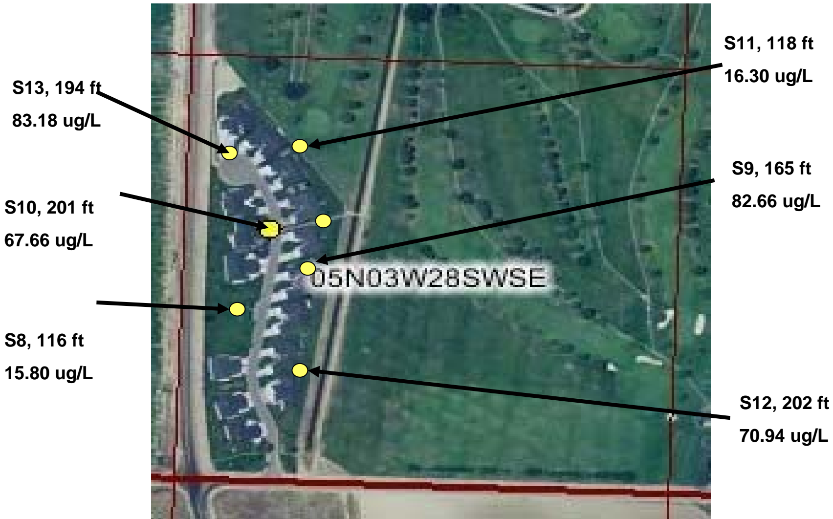
Figure 32. Group 1 well locations shown by aerial photo. Labels show well depth (ft below land surface) and uranium concentration ( \mu\text{g/L U} ). The six wells are located within the same quarter-quarter section (40 acres) which is \frac{1}{4} mile square.
