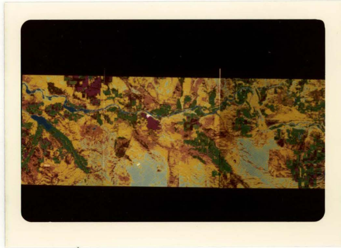
Figure 8. DICOMED output of computer classification of the Western Test Site using September 1974 data. Various green and purple areas represent irrigated cropland.
