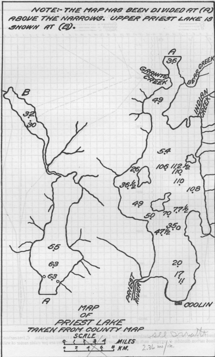
FIG. 17.—Map of Priest Lake and Upper Priest Lakes locating soundings. The depths are given in meters.
