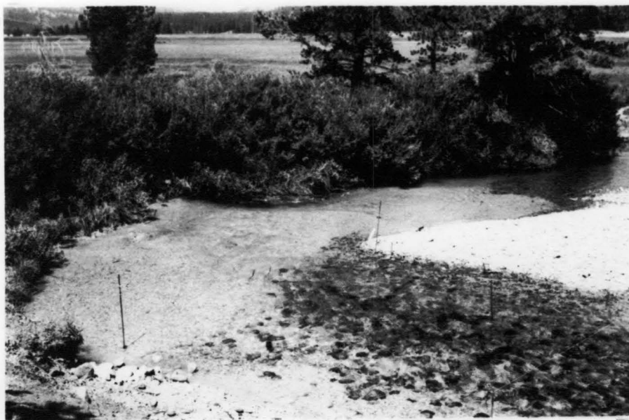
Plate 5. The main pool in the Knapp Creek test section after the second addition of sediment and just prior to the last addition of sediment. (looking downstream)
