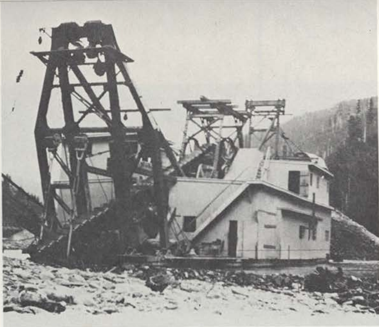
Huge dredge operating on Pritchard Creek was capable of removing placer gold beneath twenty-five feet of coarse gravel and boulders.
