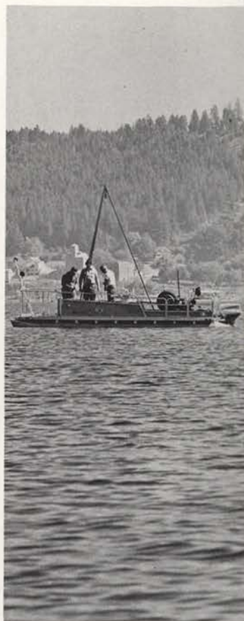
Washington State University research barge was used to obtain cores of bottom sediments of Coeur d'Alene Lake. Study of such cores reveal water quality trends.
