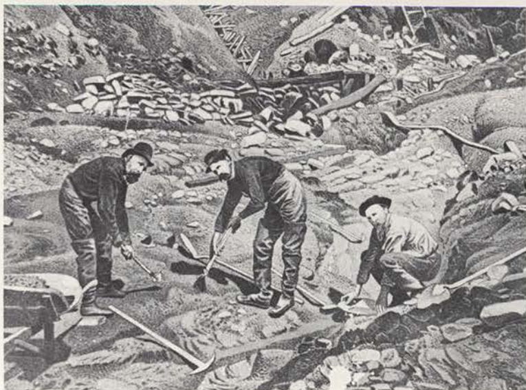
Early placer miners used a pick, shovel, and pan to search for gold.
