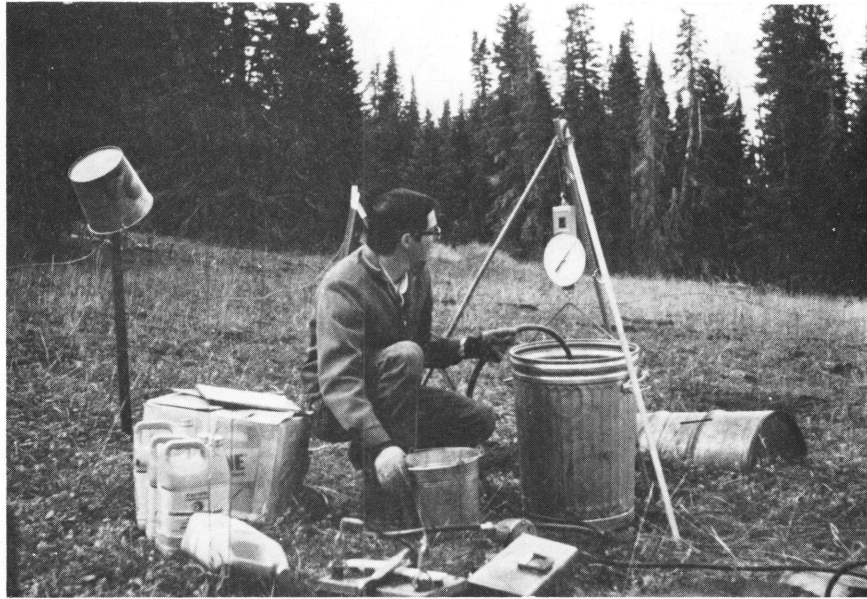
Figure 14. Graduate Student, David Fortier, pumping out the 55-gallon "drum gage" at the Clear Creek Meadows site.
