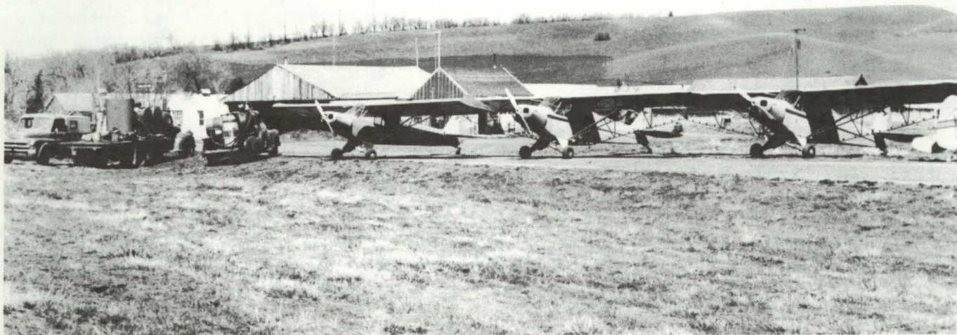
A pick-up and a truck, both with chemical tanks ready to fill the waiting hoppers of a Piper J-3 (left) and two Piper super cubs.
