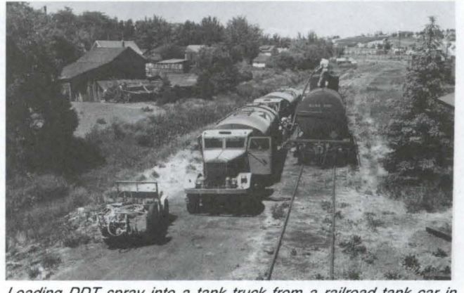
Loading DDT spray into a tank truck from a railroad tank car in Moscow for transportation to airstrips.
