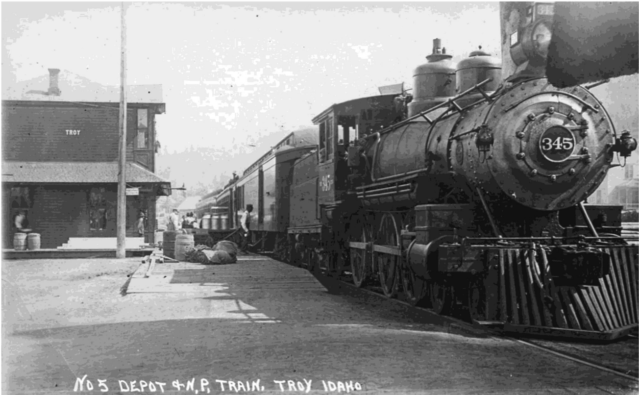
Figure 7. TOP: Howell Junction was a wood/water stop on the S&P (Courtesy of Troy Historical Society). BOTTOM: Engine #345, a 4-6-0 "Superheater" built by the Baldwin Locomotive Works in 1890, sits at the standard S&P (NP) two-story Troy depot. The station agent lived upstairs. (Courtesy of Steven R. Shook collection)
