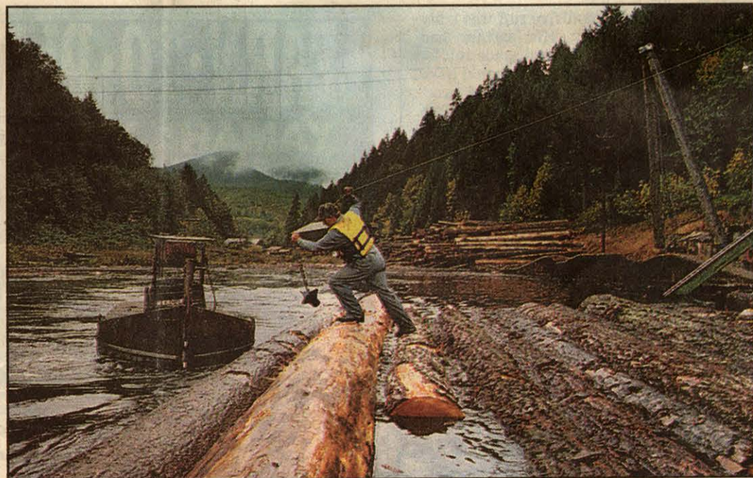
Above: For 62 years, the Hull-Oakes mill has kept the valley humming near Monroe. Left: Mike Wiard attaches a hook to a log raft to keep it tight against a gathering machine in the mill's log pond. Logs are trucked to the mill from sites in the Coast Range.
