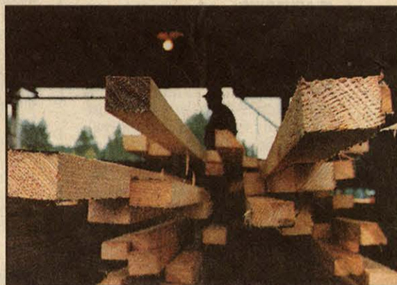
Although the mill is set up to cut large, long logs, nothing is wasted. Massive structural timbers are its specialty, but the sawyer maps out the cut to get products all the way down to spindly 2-by-2s.
