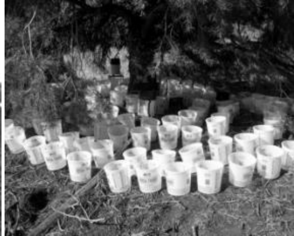
Illustration 2.3b Buckets placed under the canopy for capturing throughfall.
