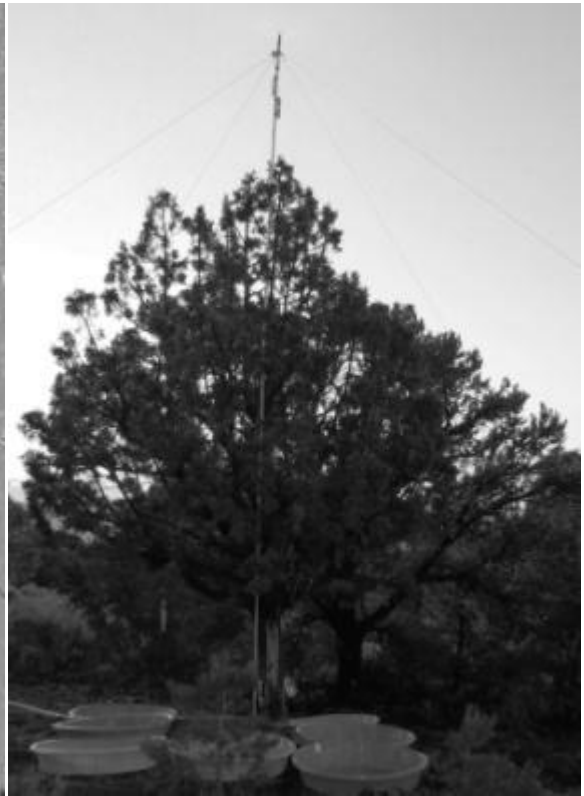
Illustration 2.1b Rainfall simulator and pools beneath the tree canopy for throughfall capture.
