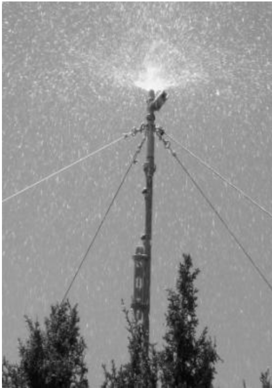
Illustration 2.1a Rainfall simulator. Note: four guy ropes, levels, pressure gauge and nozzle.
