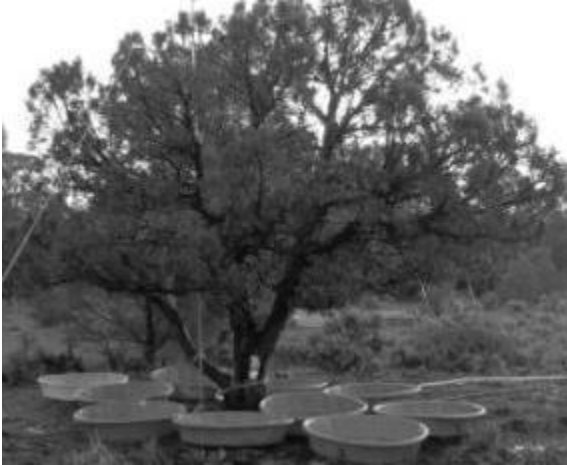
Illustration 2.3a Pools used beneath tree canopy for capturing throughfall.
