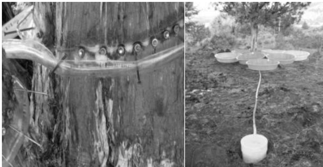
Illustration 2.2a Stemflow collar attached to trunk of tree.
