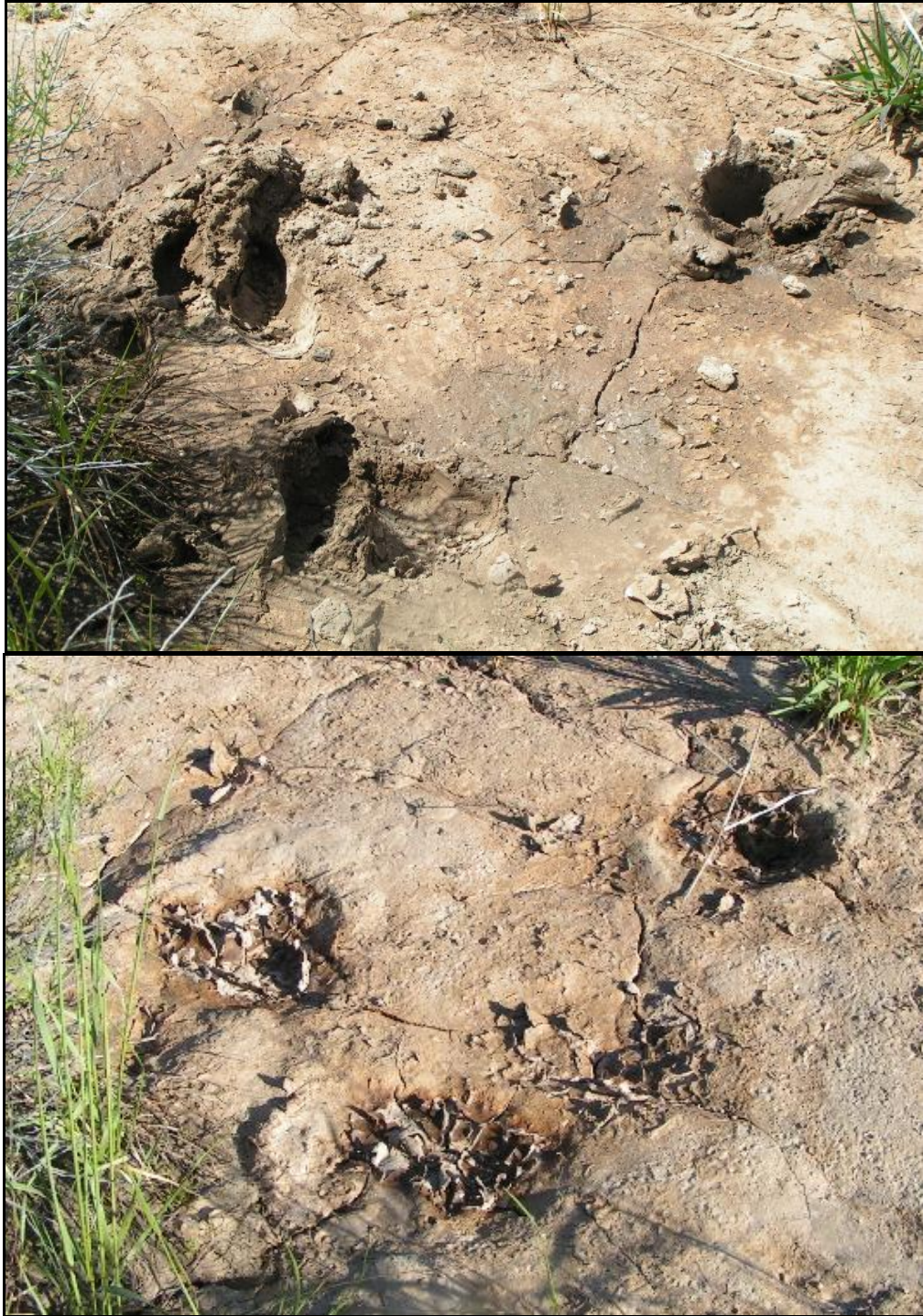
Figure 6. Silting in of hoof-prints just after 3 weeks – maximum depth on day of treatment (upper image) was 3.5-cm and 3 weeks after, 1.5-cm (lower image).
