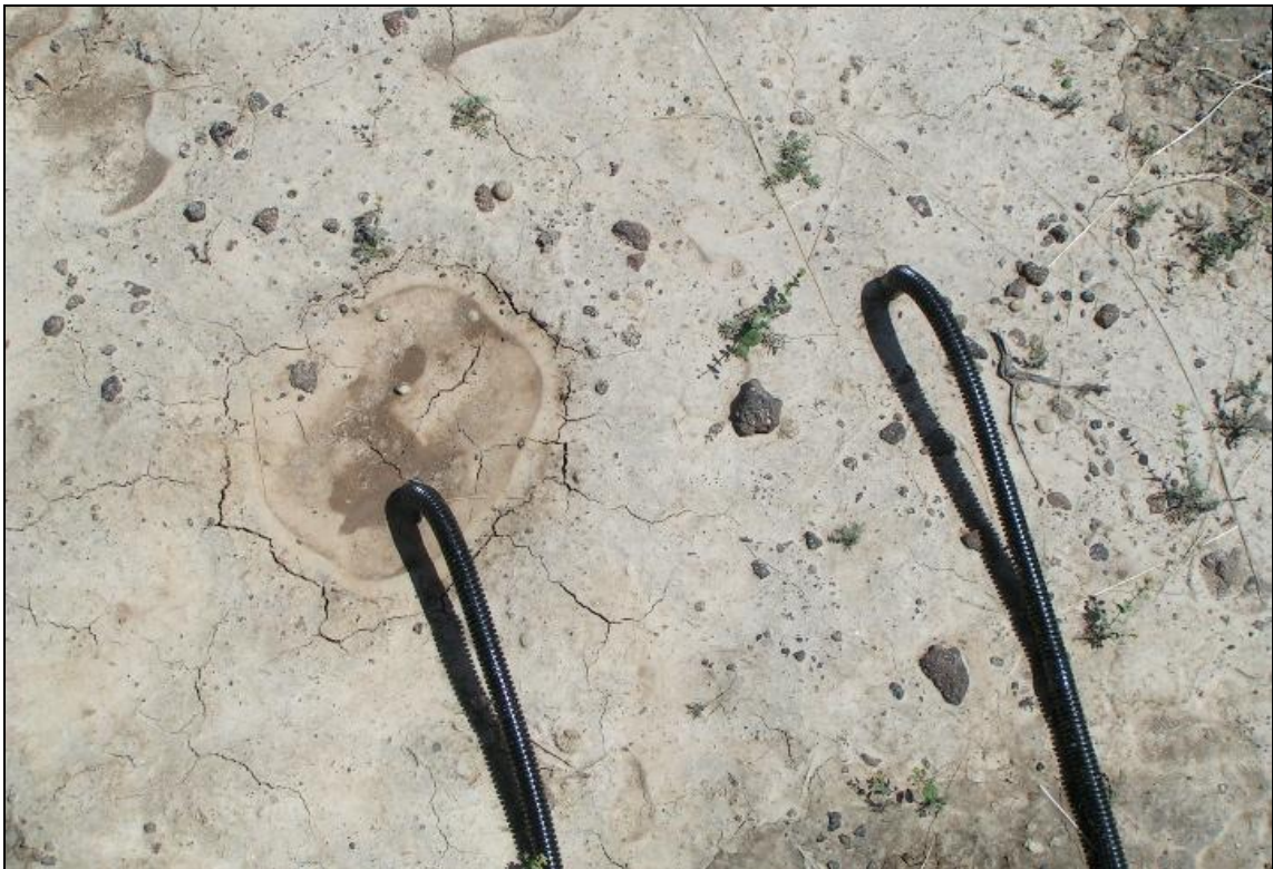
Figure 4. Example of the volumetric soil water content measurements inside and out of hoof-prints.
