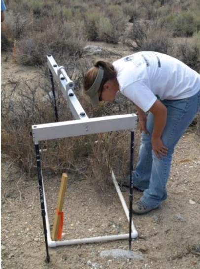
Figure 9: The laser point frame is supported by three adjustable height legs. The lasers are spaced 10 cm apart in the long portion of the “t” and point downward toward the ground.
