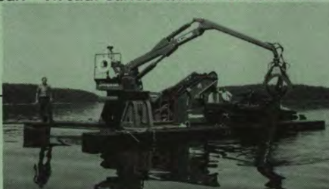
This red-clawed "Logster" is being used by Simpson Timber Co. to sweep floating debris and logs around the company's waterfront at Shelton, Wash.
