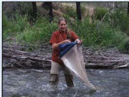
Amanda using the Surber stream bottom sampler to collect aquatic invertebrates. (right) Greg, intern, and Jess measuring stream cross section.
