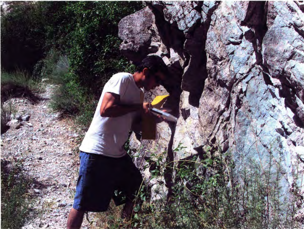
Figure 14. Photograph of the Schmidt hammer being used to measure bedrock rebound. Measurements were taken with the hammer positioned normal the surface being measured.
