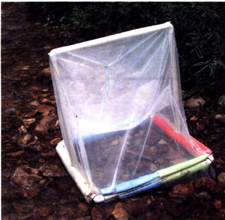
Figure 3.1. (A) Light-weight emergence trap designed for use in wilderness, or other logistically difficult settings. (B) Modified emergence trap for collection of bank emerging taxa.
