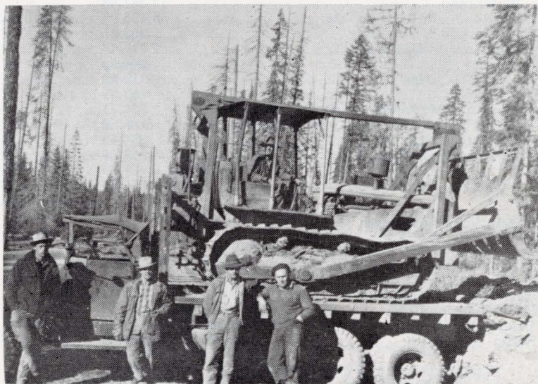
Specially designed 6x6 truck bed makes for rapid transportation of D-6 Caterpillar equipped with brush blade used for efficient piling of logging slash. Emil Keck, slash disposal supervisor, and George Space, fire warden, supervise loading job.
