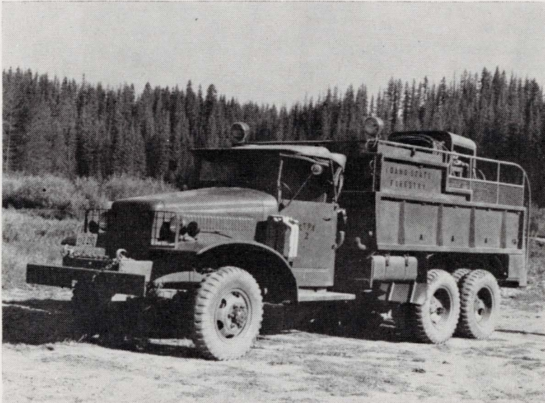
International truck powered in six wheels with tank and pumper for use on low class roads and skid trails.
