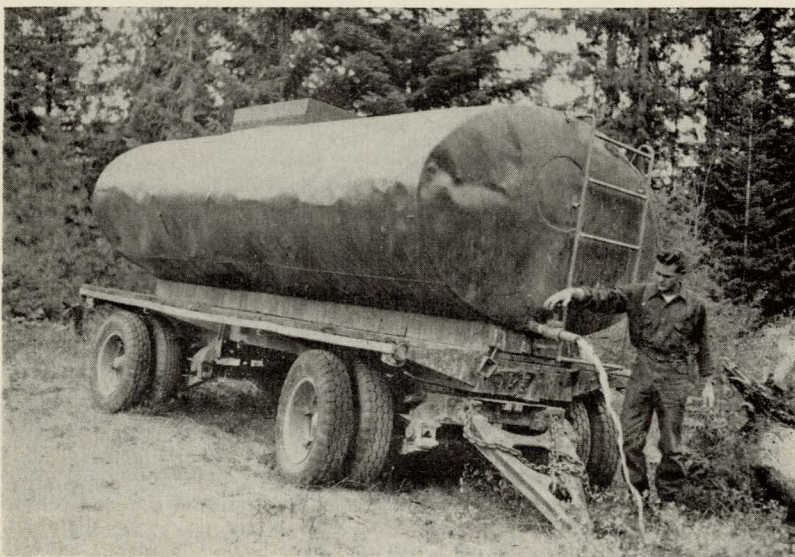
This five thousand gallon tank was salvaged from a gasoline tanker outfit which had tough luck on the highway. Instead of holding gasoline, it now sits on one of our bad fuel locations with five thousand gallons of water always ready to be used during fire season. During the fall it is emptied and put away. This is another example of intensive protection.
