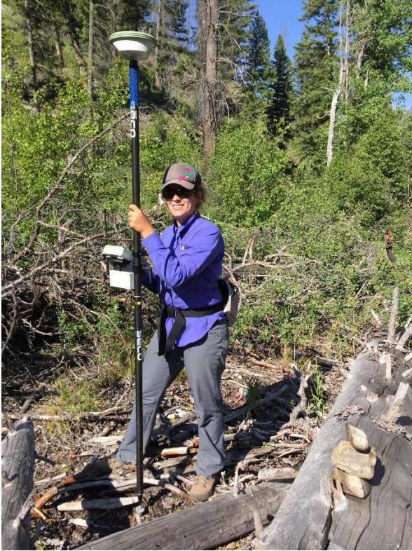
Emmy at work surveying the logjam with a RTK GPS that returns positions with a precision of <1 cm. This was used to set initial control points. Jam D surveys were completed using a total station with a precision of \sim 1 mm.
