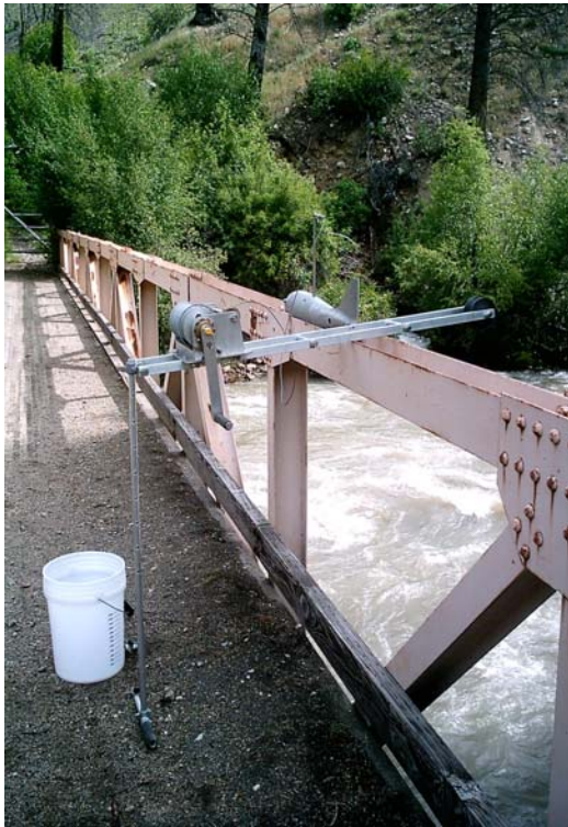
Figure 3. The isokinetic sampler used solely on Big Creek. The bridgeboard rests on the top railing of the bridge and a cable reel lowered the whale into the water column. Next to the support leg for the bridgeboard is the integration bucket.
