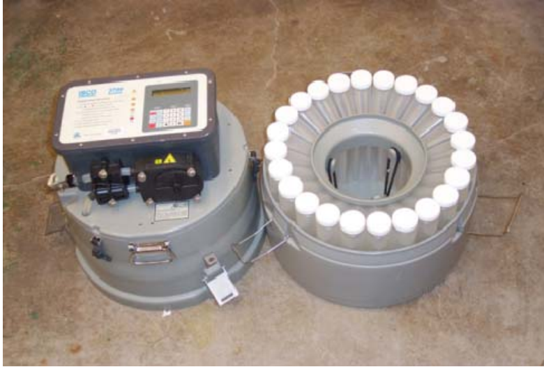
Figure 4. The ISCO sampler shown with the top section removed, exposing the 24 sample bottles. Programming the unit was done using the keypad. The top section has a weather resistant cover, not shown.
