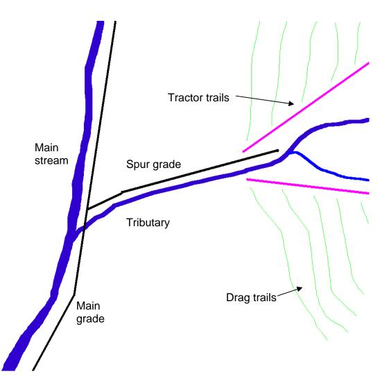
Figure 4: Diagram of surface earthwork features found on the UIEF relating to railroad grades. The spur railroad grade is a temporary grade built to move logs out of a given drainage to the main railroad grade. Tractor trails were used by tractors or possibly horse teams to move logs down slope to rail cars. Drag trails were created by dragging logs to the tractor or horse team from the harvest point.
