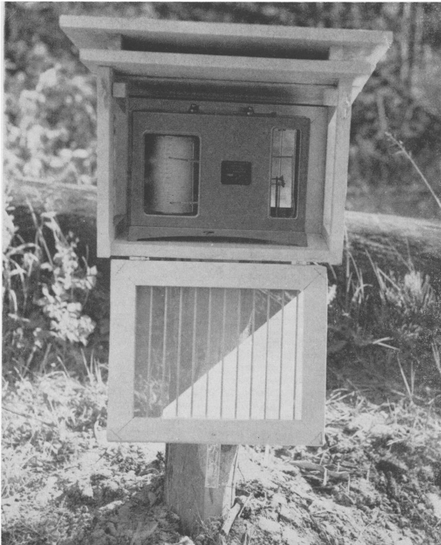
FIG. 1. Instrument shelter in use housing a hygrothermograph. The shelter here is mounted on a single post, two feet above the ground.
