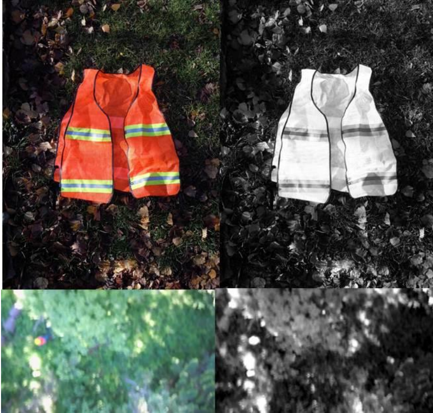
Figure 1: High visibility safety vest with no filtering (left), and with a red band filter applied (right).
