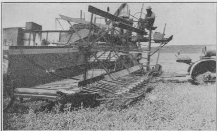
Fig. 10. A combined harvester adjusted for harvesting peas, operating near Moscow, Idaho.
