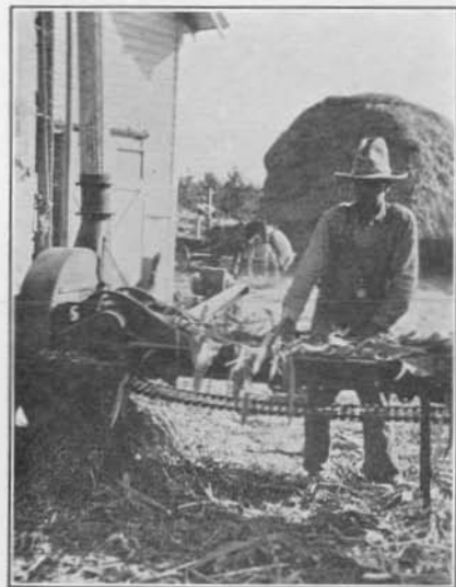
Even feeding is essential to the successful use of a 5- or 7½-horsepower electric motor for silo filling power
