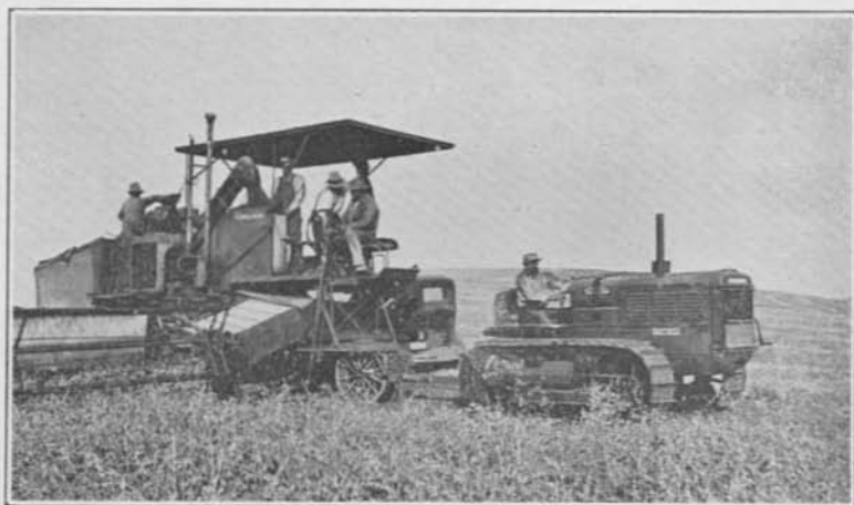
Fig. 5.—Diesel tractor, and combine equipped with special "pea reel" developed by the Department of Agricultural Engineering and local pea growers.
