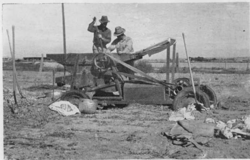
Figure 4.—Cleaning bean thresher used on the bean experiment plots. The engine, tool-box, and separator are mounted on a trailer.
