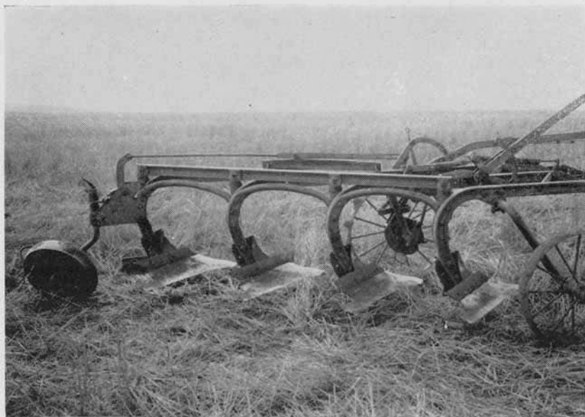
Figure 6.—Modified moldboard plow, converted from four bottom moldboard plow.
