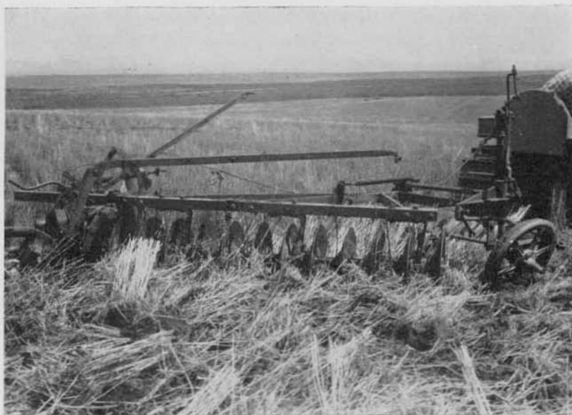
Figure 10.—One way disk working in 4,500 pounds of straw and stubble residue.
