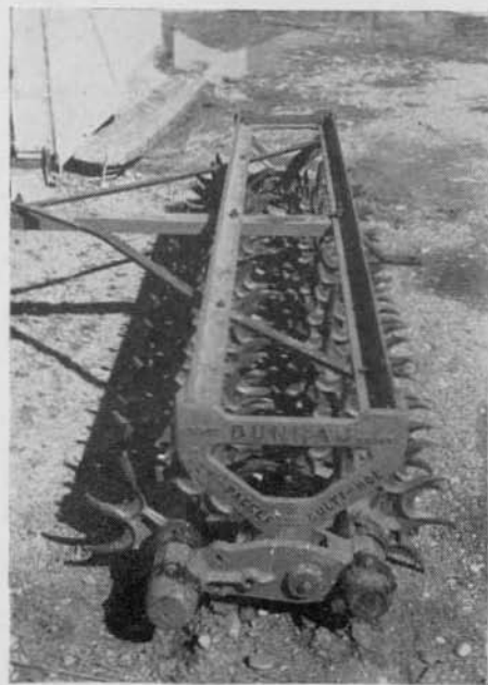
Figure 12.—Rotary culti-hoe run in reverse is used for preparing a firm even seed bed before drilling.
