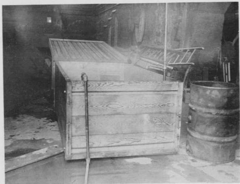
Figure 19.—Method of heating solution when steam is available. The steam passes through submerged coil, under false bottom, heating the formalin solution to desired temperature.
