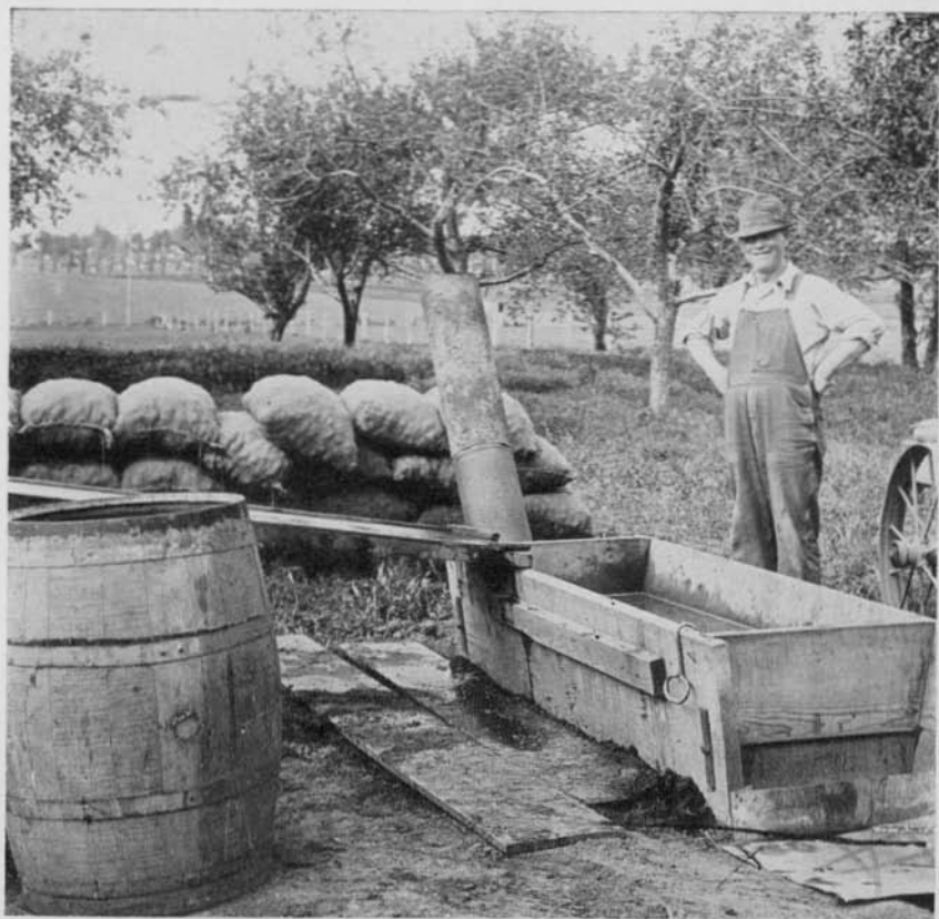
Figure 18.—One type of tank used in heating formalin solution. Plank sides, metal bottom, placed over hole in ground.
