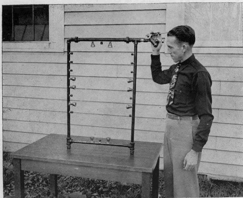
Figure 1.—Spray boom developed for treating large range bands. Nozzles arranged for best spray pattern.
