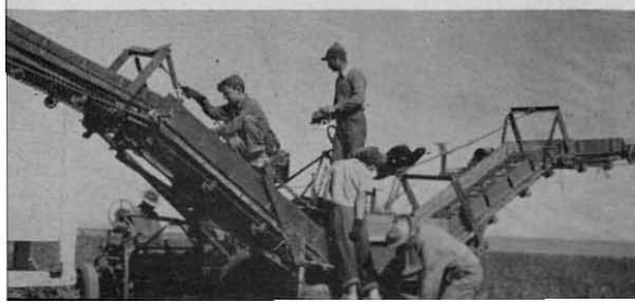
Figure 24. A bulk harvester with specially built elevators that enables the digger to operate on adjacent rows.
