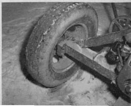
Figure 14. Close-up showing method of attaching the axle to the wheels and of mounting the small engine.
