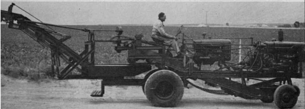
Figure 21. A self-propelled harvester using two engines. One engine to move the digger and the other to operate the digger chains and elevator.
