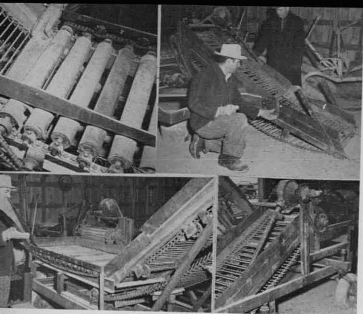
Figure 8. Single-row bulk harvester. Upper left—rubber separating rolls mounted across the rear of the machine. Note the method of driving the rolls and rubber belting used to protect the potatoes from injury. Upper right—the digger point mounted under the tractor. Lower left—the rubber separating rolls. Note the relation of the digger chain to the roll assembly. Dirt separation takes place over the rolls and the potatoes are moved to the elevator and into the truck. Lower right—view showing the digger chain, caster wheel and power take-off drive.
