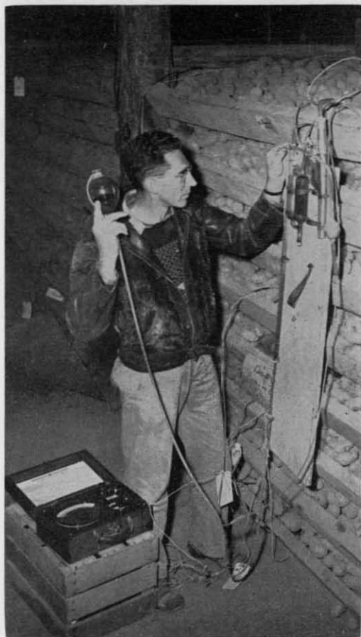
Figure 13.—Storage studies with potatoes. Walter C. Sparks, Horticulture, checks circulation of air by means of gas analysis in a bin of Russet Burbank potatoes at the Aberdeen Branch Station.
