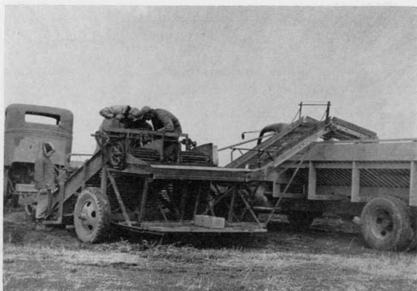
Figure 17.—The two-row light-duty bulk handling potato harvester ready for field operation.
