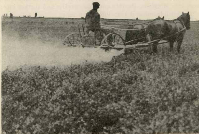
Traction Dusting Machine in Operation in an Alfalfa Field
