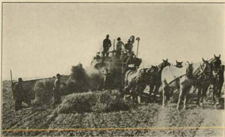
Fig. 2—The semi-stationary use of the combine reduces labor and minimizes loss of peas by shattering.
