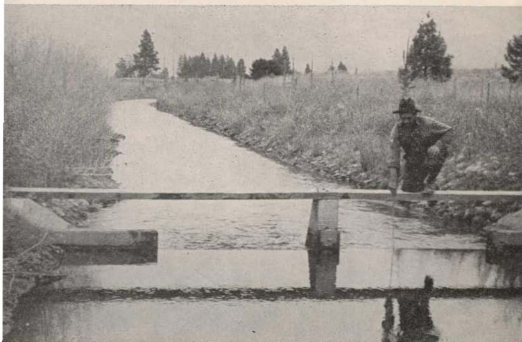
Figure 6.—The operator is measuring the water over a double rectangular weir by the "pile-up" method. This method is not recommended due to the difficulty in getting an accurate head reading. Rather, the head should be measured in still water away from the weir notch.
