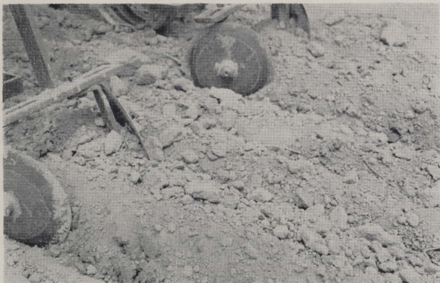
Figure 2.—A close-up of the "hiller" attachments used to ridge soil on the rows.
