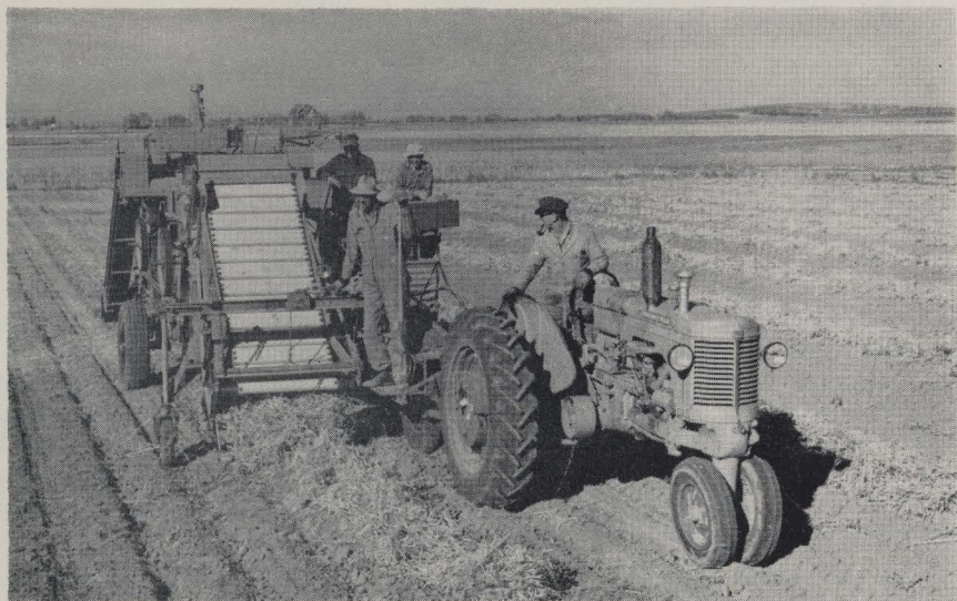
Figure 3.—C. B. Hay bean harvester at work in southern Idaho. This is one of the more popular types of special bean harvesters used in the area. Photo courtesy Associated Seed Growers, Inc.
