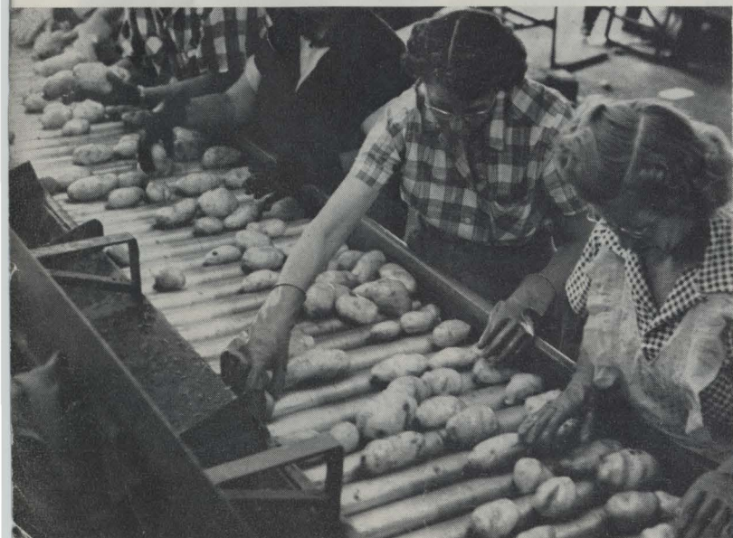
Figure 1—Potatoes revolve as they move forward. No hand turning of potatoes.
