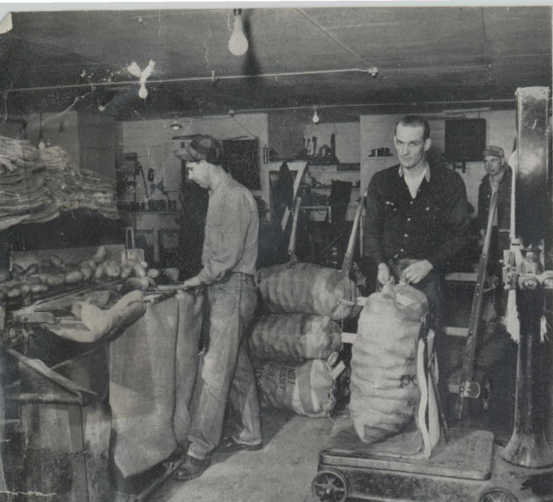
Figure 22—Jigging and sewing 100-pound sacks. This is the common way of filling burlap.
