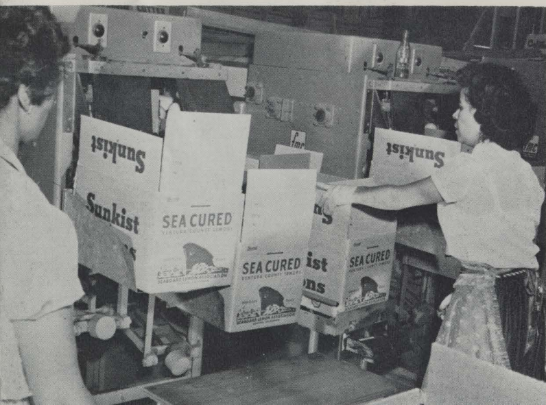
Figure 4—Semi-automatic box filling machine. This type requires one worker for each machine.
