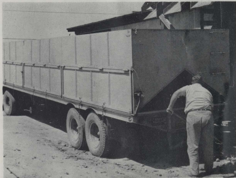
Figure 11—Cull truck holds 20 tons. Doors permit emptying on either side.
