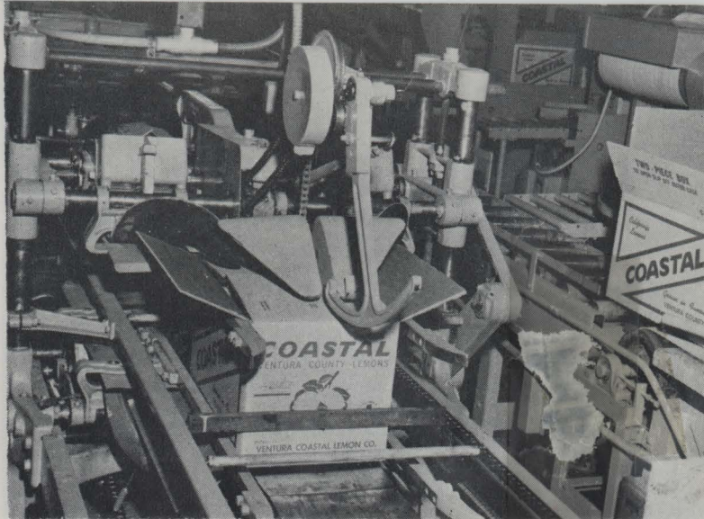
Figure 5—Box lid being closed automatically.
