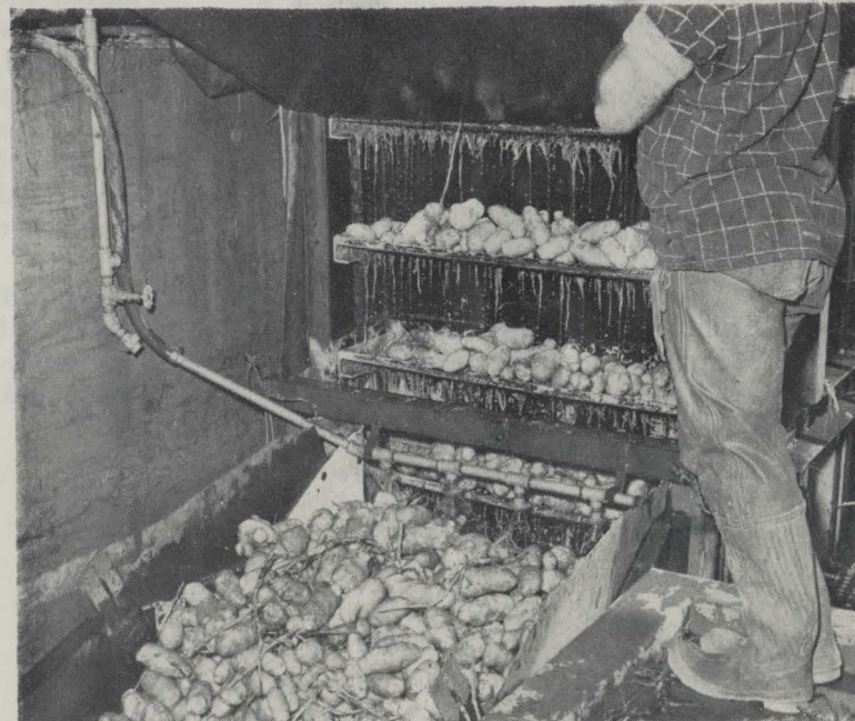
Figure 24—Vertical elevator takes little floor space.
