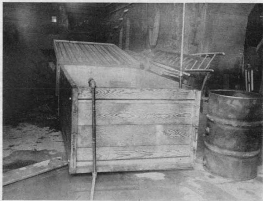
FIGURE 18.—Method of heating solution when steam is available. The steam passes through submerged coil, under false bottom, heating the formalin solution to desired temperature.
