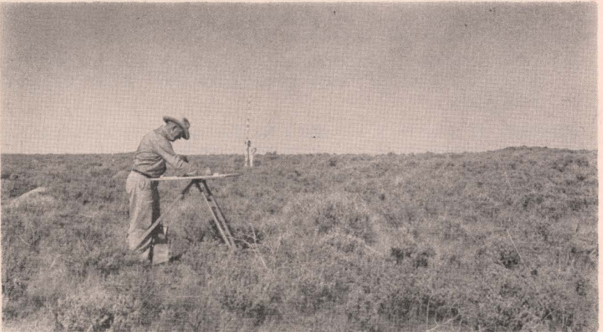
Figure 2.—Plotting a contour map is the first step in developing desert land. This southern Idaho farm was planned with the assistance of the Soil Conservation District.
