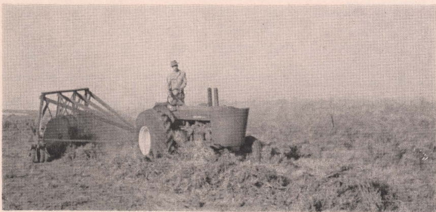
Figure 3.—Brush is windrowed for burning after it was cut with a blade.
