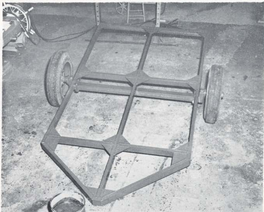
Figure 1.—The all-steel welded frame construction. Note the axle mounting method used to lower the frame. Holes are provided in the frame so the axle may be shifted forward or to the rear to obtain the correct balance of the trailer.
