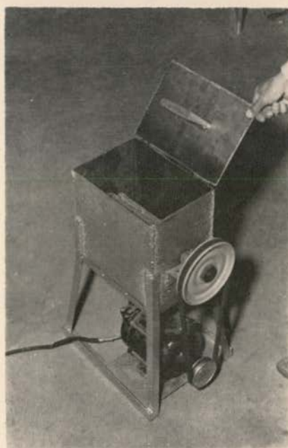
Figure 1. Left—Photograph of artificial bean seed injury machine developed by the Associated Seed Growers.
