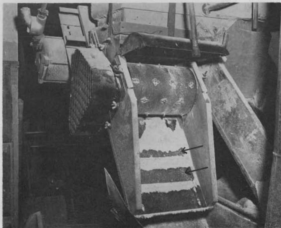
Figure 11 — Front view of the machine showing drum and magnet as installed in the chute. Arrows point to the pole faces of the magnet.
