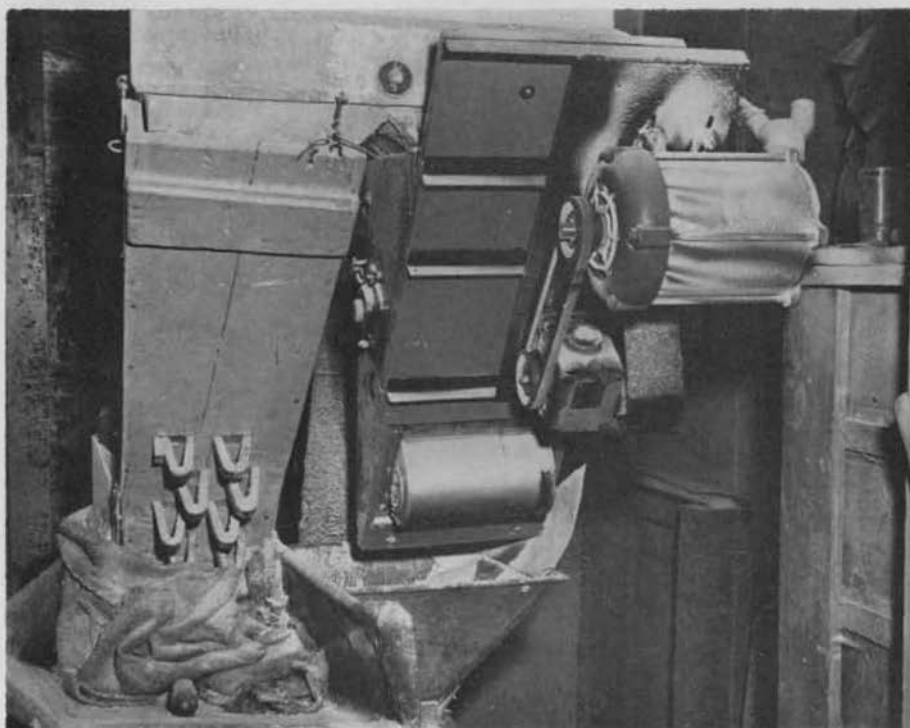
Figure 13 — Rear view of machine showing motor mounting, belt arrangement, and gear reduction unit. The magnet can be seen at the lower part of the chute. The other chute shows an old installation using U-shaped magnets. These have become demagnetized and are of little value.
