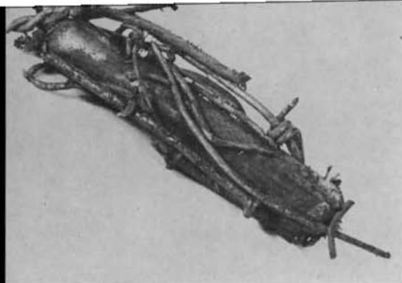
Figure 1 — An Alnico bar magnet covered with tramp iron as recovered from the stomach of a cow by the Department of Veterinary Science, University of Idaho.
