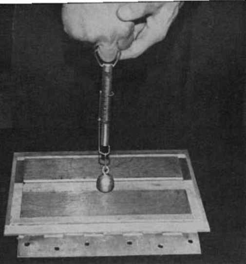
Figure 6 — Measuring the holding-power of a plate magnet.
