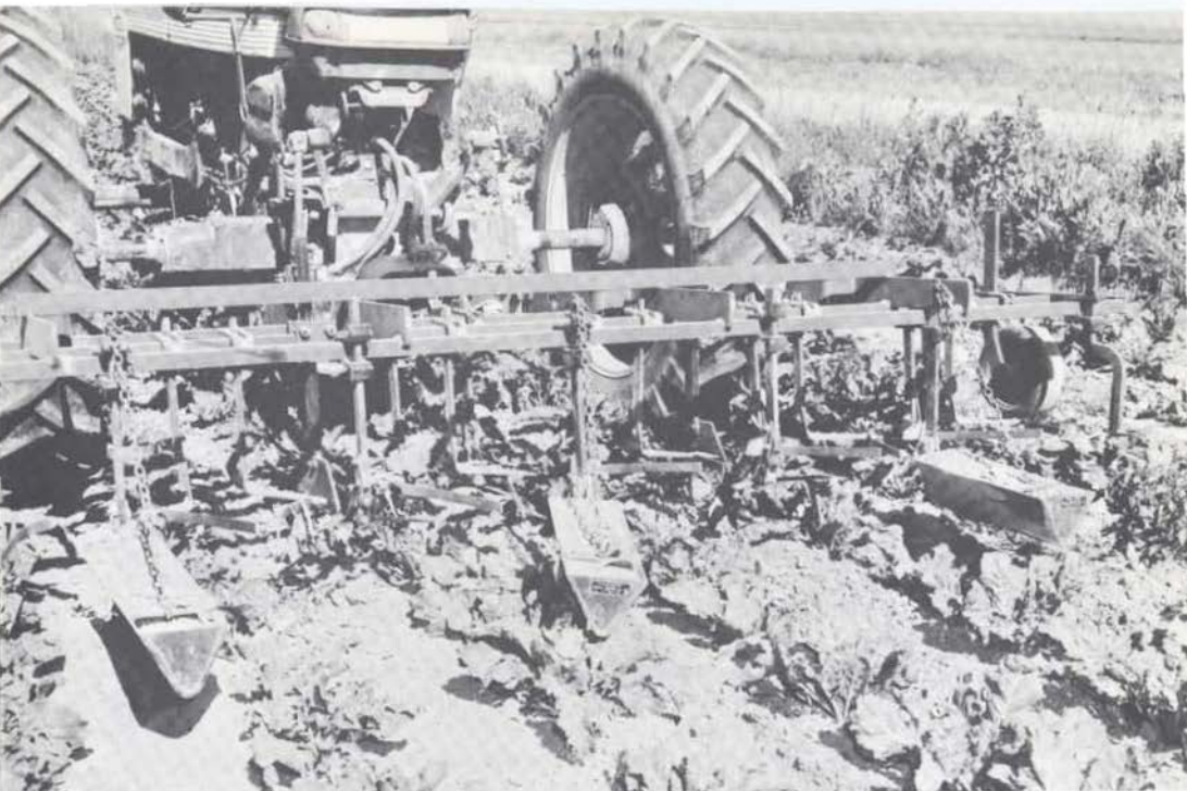
Figure 6. The assortment of cultivator tools ahead of the slickers controls weeds, and provides a loose, clodless, free-flowing soil for the furrow slickers. The furrows are re-slicked after each cultivation.
