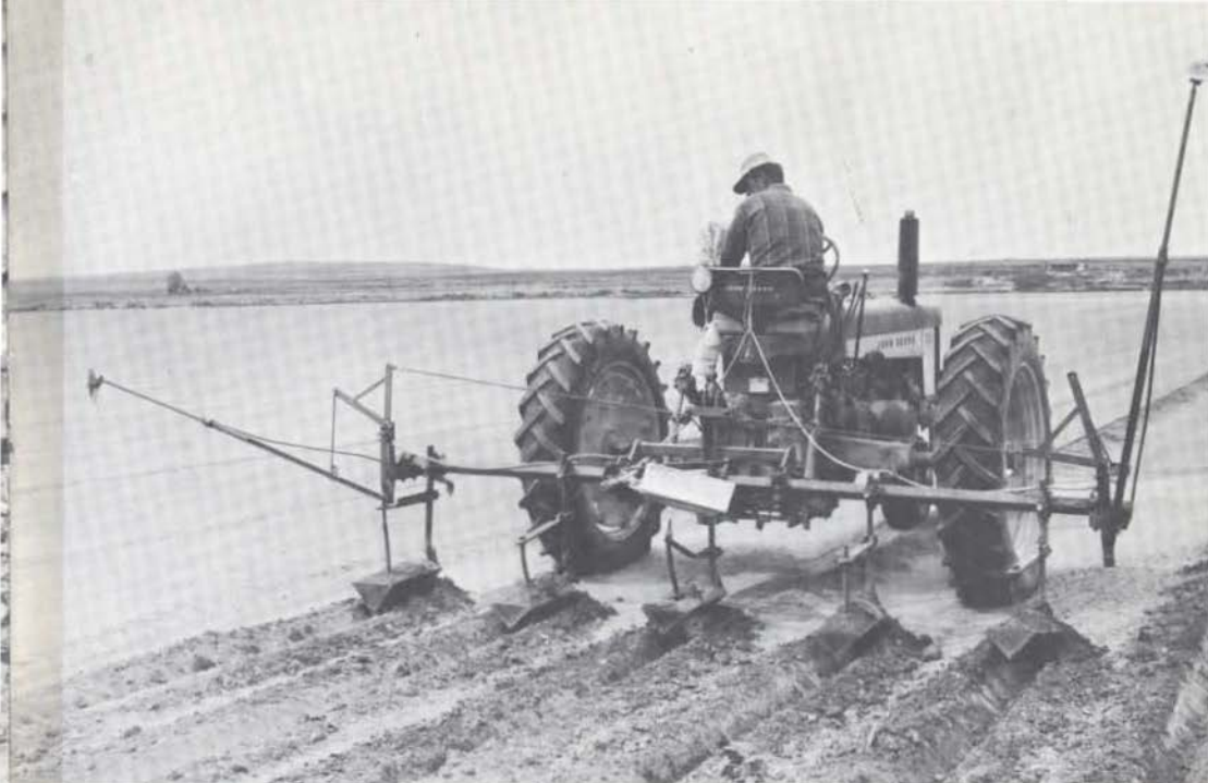
Figure 2. The field is marked out and corrugated for irrigation before planting beans. The marker is followed easily by the tractor. Slick furrows allow a light, uniform application of water. A light irrigation permits the soil to be worked sooner and an earlier planting.
