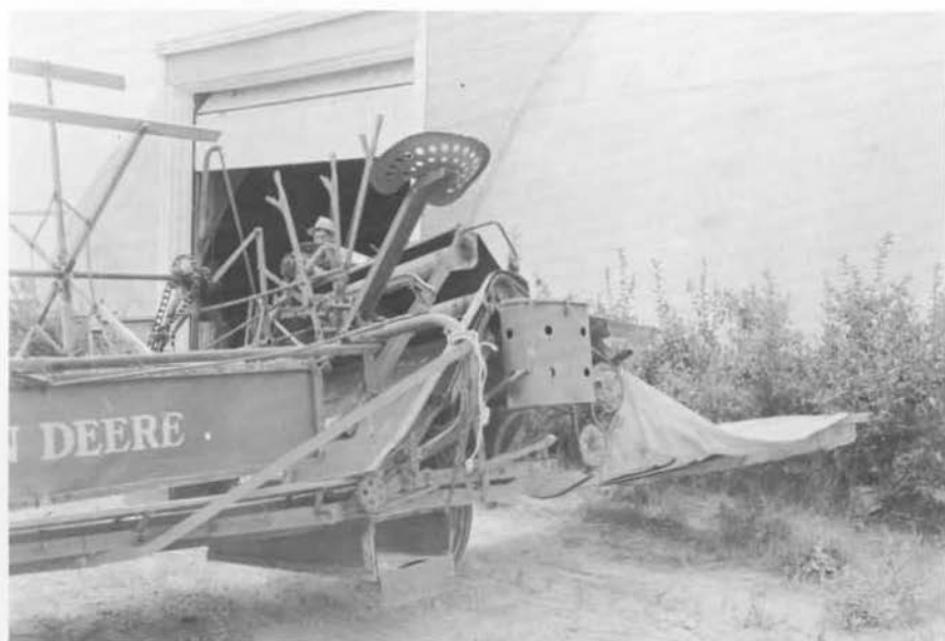
Figure 1. A binder equipped with a metal catch pan beneath the roller and with a canvas over the bundle rack catches seed that shatters during the binding operation.
