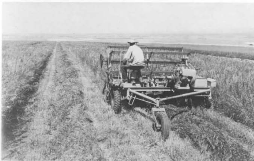
Figure 2. A self-propelled swather can be used advantageously for harvesting seed of some grass species.
