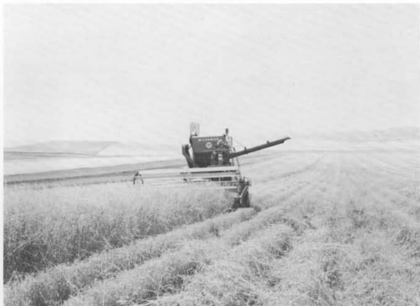
Figure 3. Direct combining is the easiest method of harvesting grass seed, but the seed must be ripe before this method can be used.
