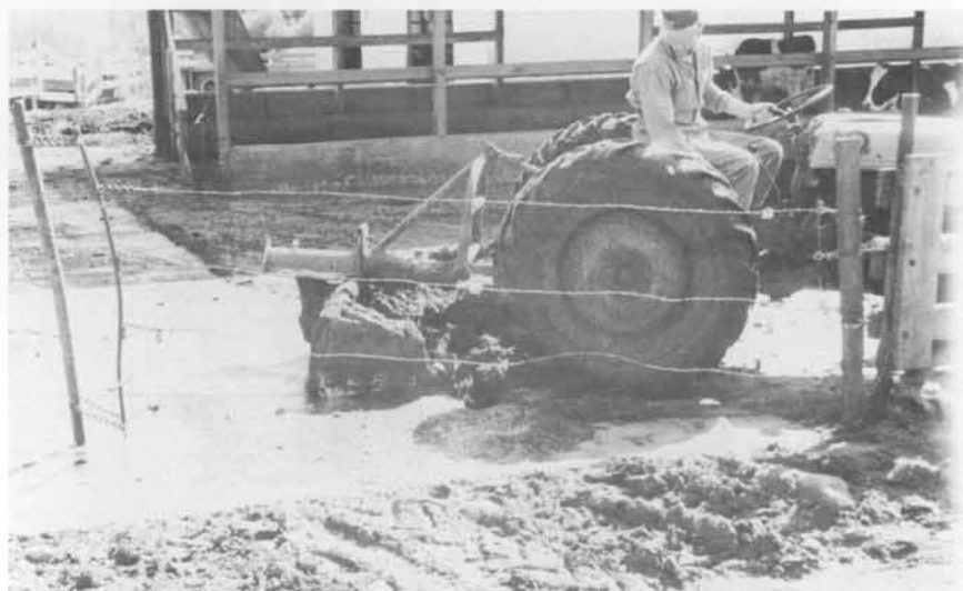
Figure 7. A tractor scraper similar to this one may be used to fill the tank or to supplement a mechanical barn cleaner.
