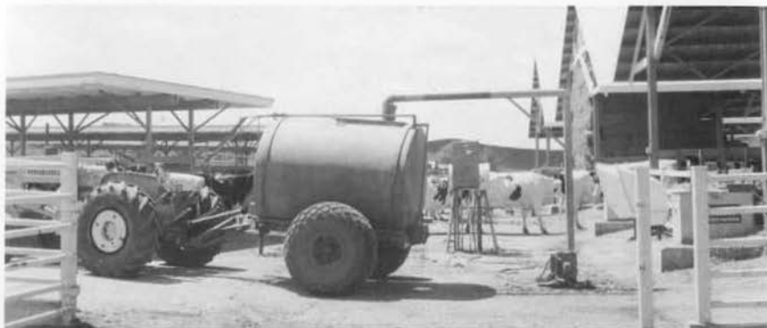
Figure 1. Complete system includes storage tank, pump, spreader tank and method for filling the storage tank. Tractor and scraper can replace or supplement a mechanical barn cleaner.
