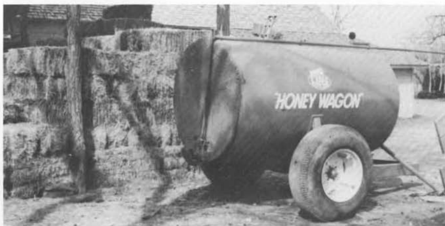
Figure 9. A combination tank wagon and vacuum pump. The tank is filled by its own vacuum pump and is emptied under pressure from the same pump. The only additional equipment necessary is an agitator in the pit.
