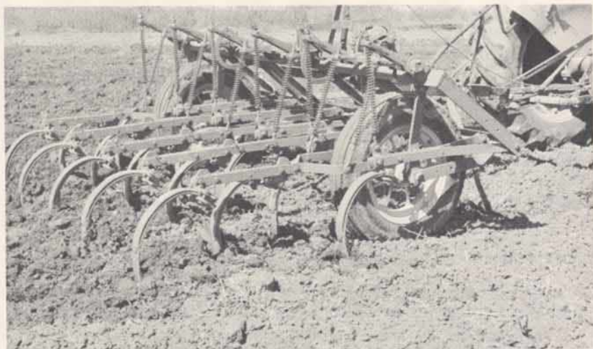
Figure 3 —A field cultivator of this type has proved to be a very effective implement for bringing quackgrass rhizomes to the soil surface. Note rhizomes on the surface in the foreground.
