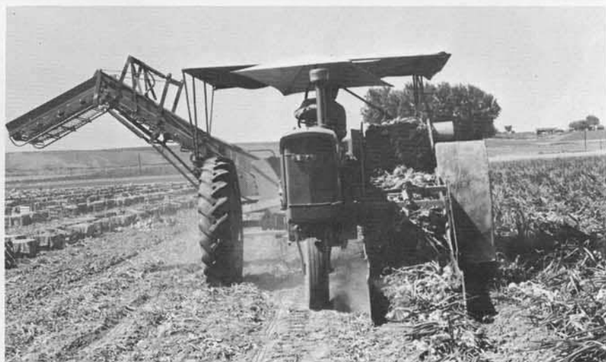
Figure 10. A potato harvester used in conjunction with the flail topper (1963-64) to pick up the topped onions.
