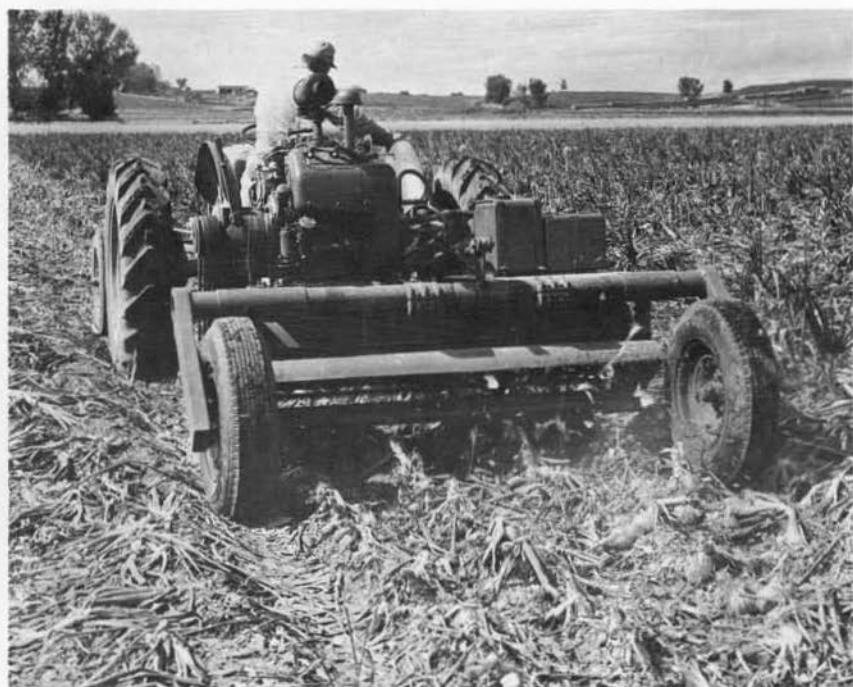
Figure 11. The flail topper designed by the Agricultural Engineering Department, University of Idaho, in use during the 1963-64 season.
