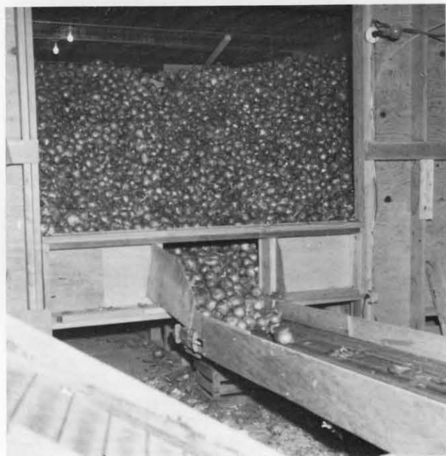
Fig. 12. Space limitations made it necessary to load and unload onions at a right angle to the truck. This required an extra cross-conveyor for unloading.
