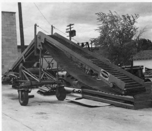
Fig. 13. This hydraulically operated piler was constructed by Parma Water Lifter Company and furnished by the Southwestern Idaho Onion Growers Assn. for use in the bulk handling experiment.
