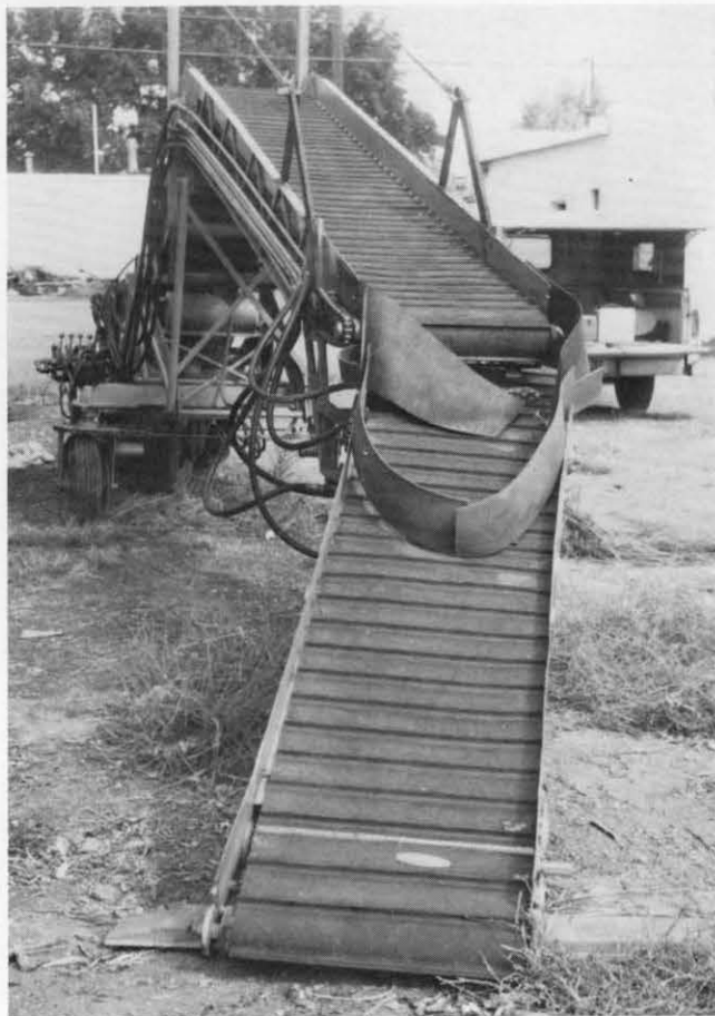
Fig. 14. An 8-foot extension distribution conveyor, added to the hydraulically operated piler for the 1966-67 experiment, was helpful in reducing onion damage.
