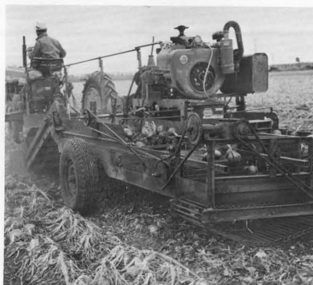
Fig. 6. The Russell topper uses a separate topping unit for each bed before windrowing.
