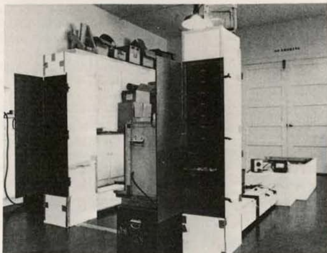
Fig. 3. Model tray dryer used to simulate a conventional hop kiln.
